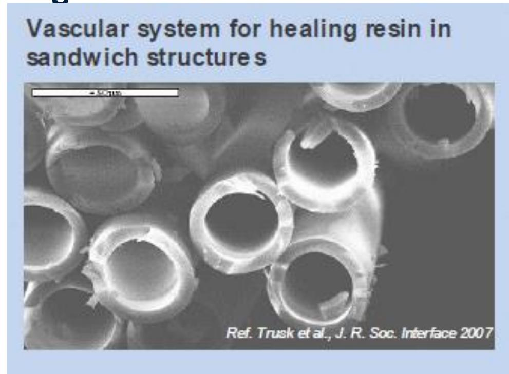
**Self-healing ability in visionary aerospace composites is able to reduce the inspection efforts and provide rapid repair**
