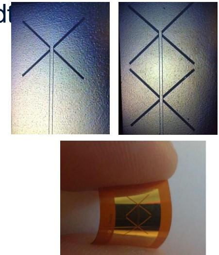
Major advantage of flexible substrate integration : facility to deploy the WSN nodes for any application
