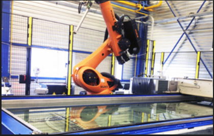
Composites inspection using SAUL
