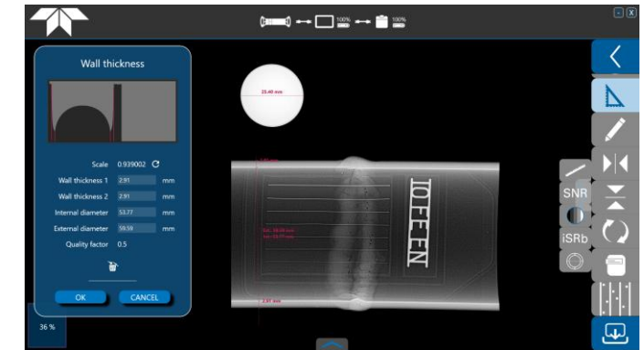
Wall thickness measurement
