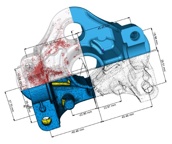
Volume Graphics software offers the ability to display and analyze both voxel and polygon data within a single application. This is because our applications also support other 3D-file formats such as point cloud, mesh, and CAD (native CAD formats and PMI with optionally available add-on modules). There's no more need for time-consuming data conversions.
