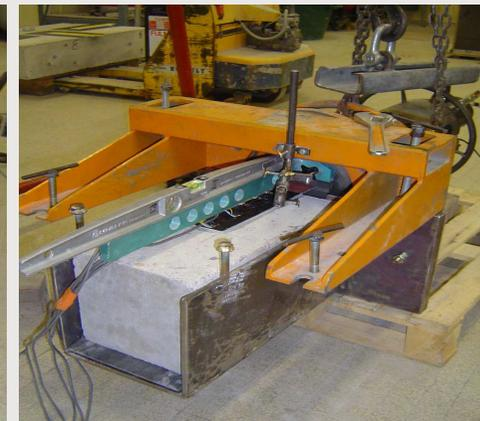
S. Chataigner, J.F. Caron, K. Benzarti, M. Quiertant, C. Aubagnac, « Characterization of composite to concrete bonded interface – Description of the single lap shear test », *European Journal of Environmental and Civil Engineering*, Vol.13: 1073-1082, 2009.
